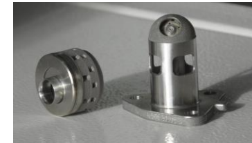
Safran combustor swirler and fuel injector nozzle
