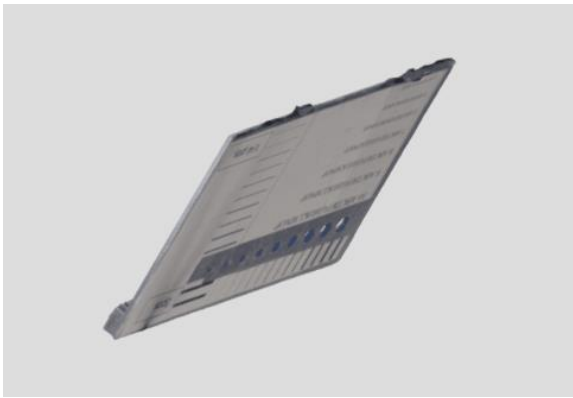
Color texture captures fine details (e.g. print lines) that geometry can't.
