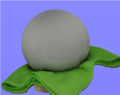
Color texture captures fine details (e.g. print lines) that geometry can't.
