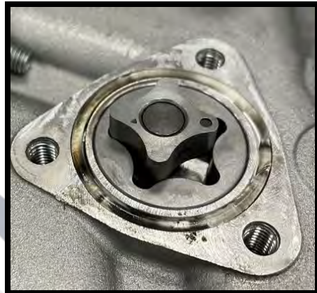
AM O-rings have different material properties (including swelling) but can be effectively used in engine applications.
