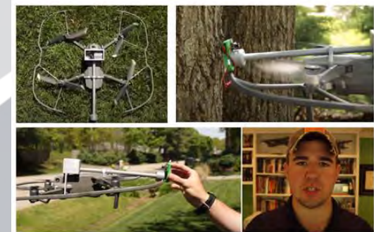
Sensor Delivery Apparatus (SDA) custom made for a UAV drone for the Service Academy Design Competition AY2021
