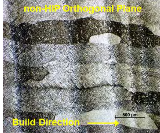
Nickel superalloy (left) and Ti64 (right) microscopy showing clear layer effects in AM structures.
